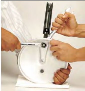
REMOVING SAFETY VALVE: VIEW OF UNDERSIDE OF LID
